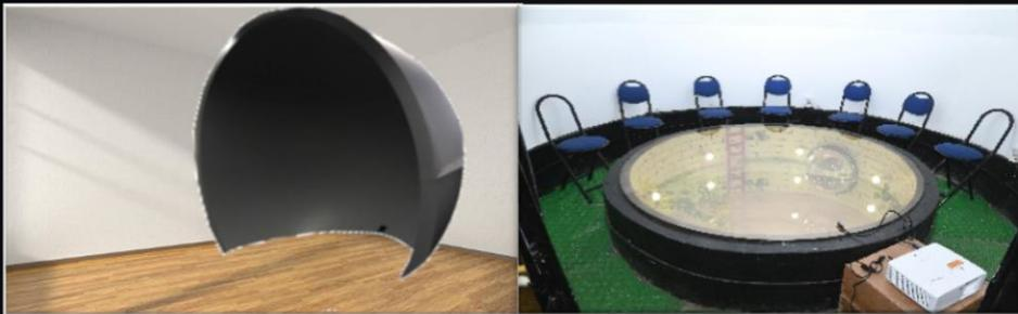
A Curve Screen (Dome), constructed from sunboard, can be installed in the corner of room/hall. At its base, a spherical mirror projection system used for the dome display. This setup is mobile, cost-effective, and offers various applications, including:
